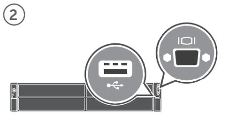
2 Connect the keyboard, mouse, and monitor (optional). 连接键盘、鼠标和显示器（可选）。 Hubungkan keyboard, mouse, dan monitor (opsional).
